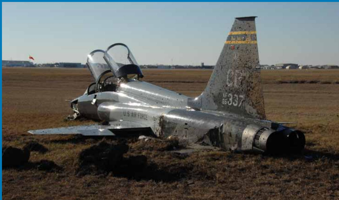
*When he became disoriented and misjudged the runway, a pilot with the 14th Flying Training Wing at Columbus AFB, Miss., crashed a T-38 Talon at Ellington Field, Texas. The crash landing caused \$2.1 million in damage to the landing gear, engines, right wing and tail section of the twin-engine supersonic jet.*
