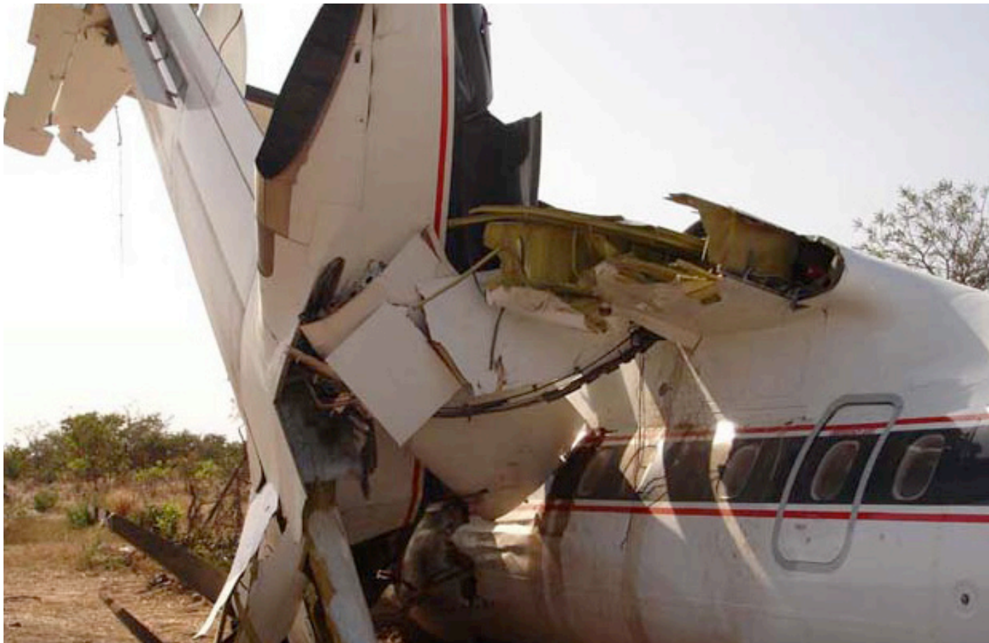
This Air Force special operations Bombardier DHC-8/Q200 crash-landed in a remote area of western Africa when it ran out of fuel and both engines shut down. All three crewmembers and six passengers were injured, with one passenger sustaining serious injuries. The $7 million aircraft was a total loss.
