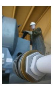
A pipe frosts over as Staff Sgt. Richard Hill works the valves on a liquid nitrogen cart. Liquid nitrogen reaches -321 degrees Fahrenheit.
