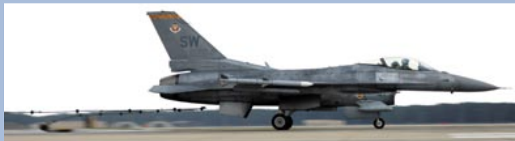
A hook on an F-16 Fighting Falcon catches the aircraft arresting system cable as part of a system test March 31.
