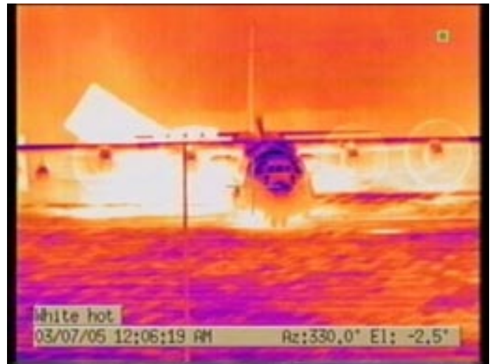
Frame 4: Twelve seconds in, the matting airfoil has collapsed with large sections blowing off.
