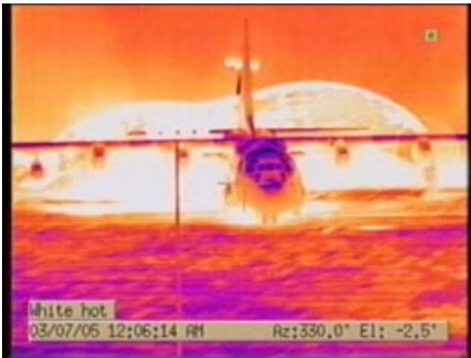
Frame 3: Eight seconds in, the matting has shifted back and knocks over a light pole behind the aircraft.
