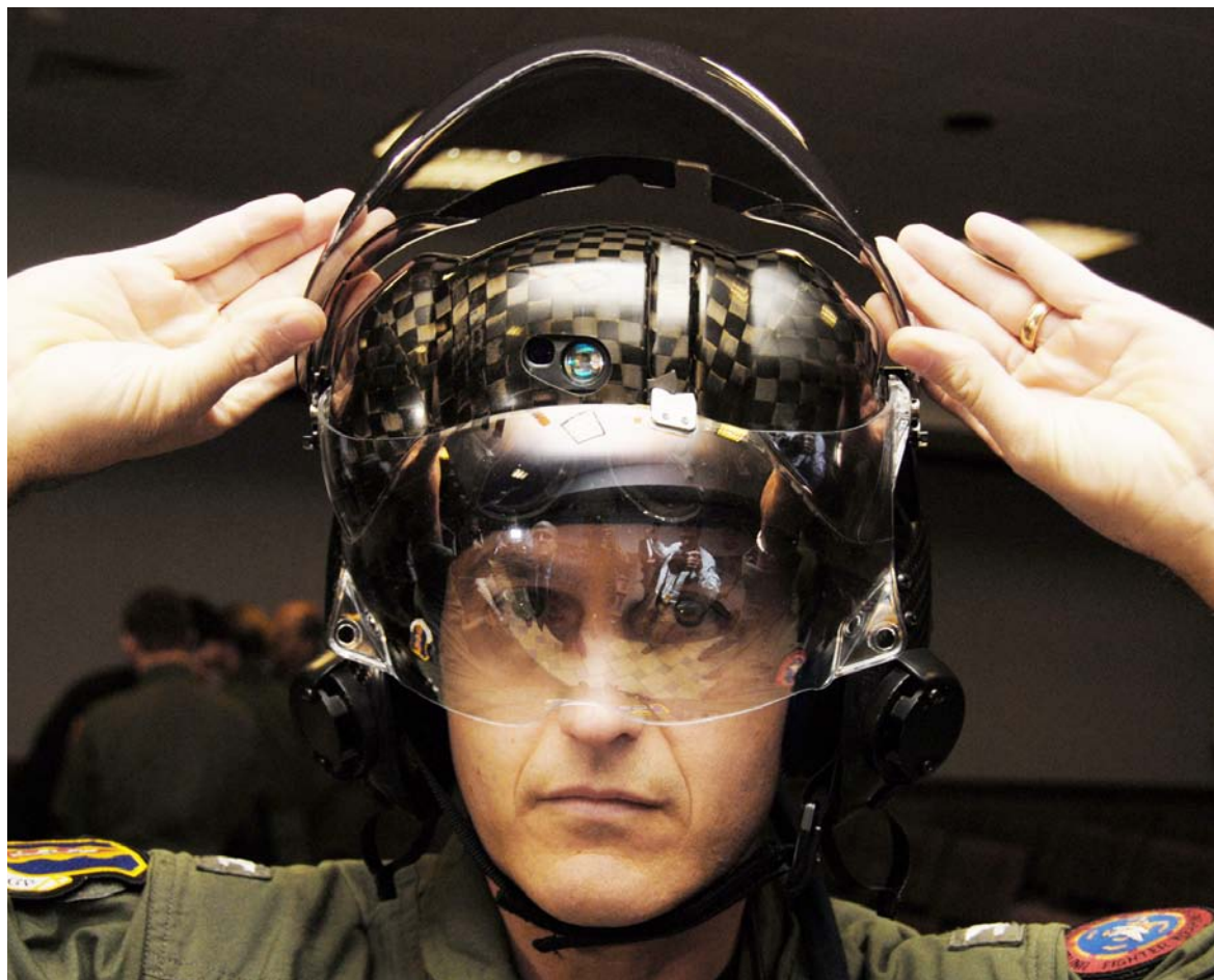
After getting measured for his new flight suit, Navy Capt. Mike Saunders, 33rd Fighter Wing Operations Group deputy commander, tries on the new F-35 joint strike fighter helmet Feb. 25 at Eglin AFB, Fla. The helmet, made of carbon fiber and Kevlar, features cameras equipped with night vision and a display system capable of projecting information such as airspeed onto the pilot's visor.
