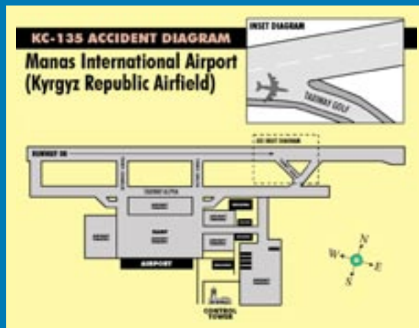
This general diagram of the Manas International Airport (Kyrgyz Republic Airfield) shows the approximate location of the control tower in relation to Taxiway Golf, as well as the approximate location of the KC-135 (inset diagram) when it was struck by a commercial aircraft Sept. 26. This diagram is based on an investigation completed by an Air Mobility Command accident investigation board.
